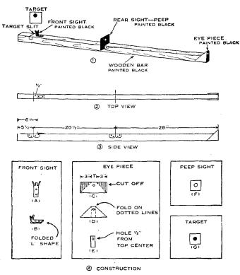
FIGURE 29.—Construction of sighting bar,
